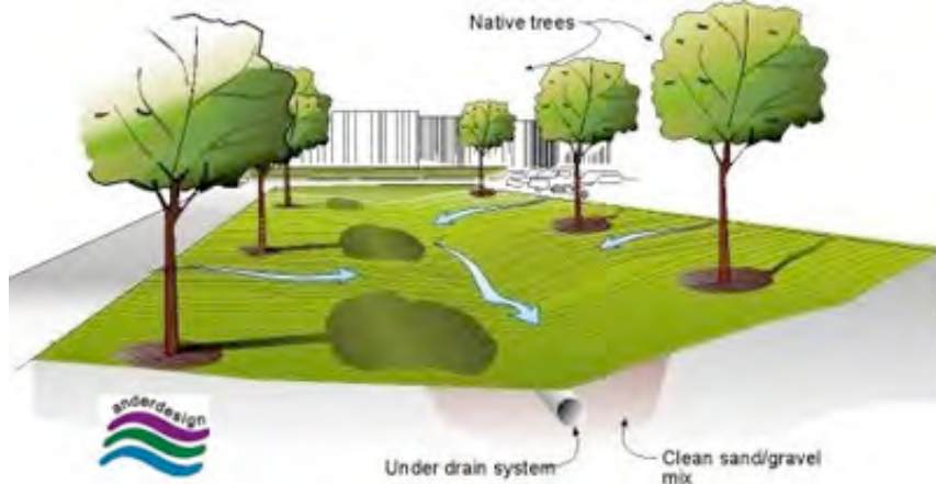
Figure 4: Longitudinal working of a Vegetated Bioswale
